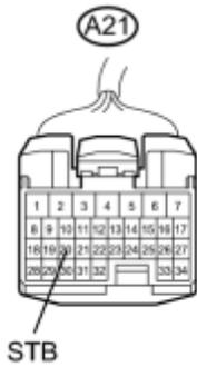
(a) Disconnect the connector from the power management control ECU.
